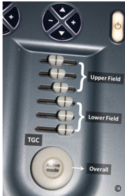
Figure 2.12: Time Gain Compensation (TGC) on an ultrasound consol. The upper and lower knobs adjust brightness in the upper and lower fields respectively (labeled). The overall knob (labeled) adjusts brightness in the whole image.
